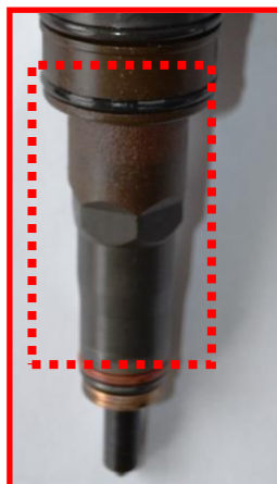
Corrosion of injector body
